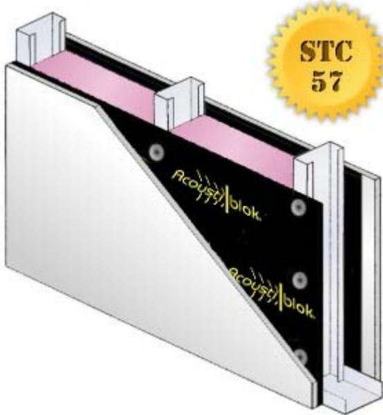
This very high performance sound blocking interior wall using two layers of 16 oz Acoustiblok adds only 1/4" of thickness and 2 lbs/ft<sup>2</sup> to a conventional steel stud and gypsum board partition. This is an example of the economy available using Acoustiblok material instead of older construction techniques: In the past, an STC 57 spec would have mandated a thicker wall and massive materials.
