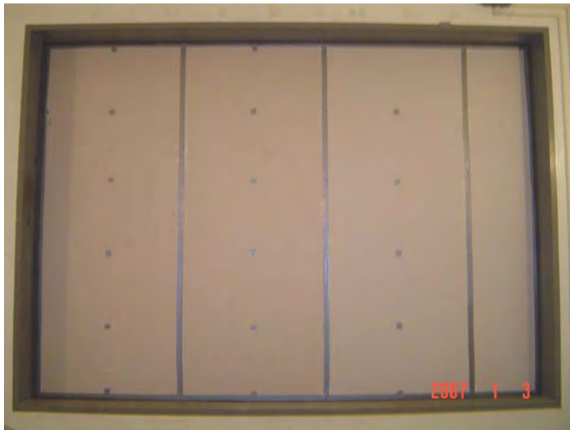
View of Specimen Installed in Source Room
