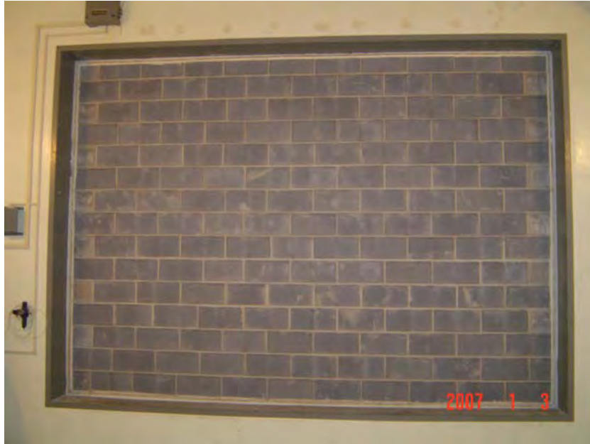
View of Specimen Installed in Receive Room
